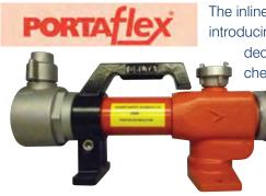
The inline inductor provides an effective means of introducing chemicals into the water stream for the decontamination, or neutralisation of dangerous chemicals or corrosive substances. The standard unit is manufactured from corrosion resistant materials and can be fixed or adjustable to deliver between 0.5 - 6% concentration. Suitable for all models in the PORTAflex® range.
