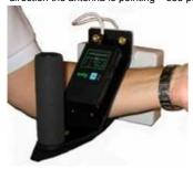
The assembly can be strapped on the officer's forearm who can then simply walk passed cells on each landing /level. The GSM196 will then indicate which cell(s) have active phones in them.
